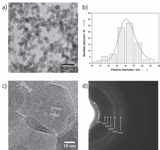
**Figure 1.** a) TEM bright-field image and b) particle size distribution of the ZIF-7 nanocrystals prepared by the excess ligand method. c) HRTEM image of the ZIF-7 nanocrystals, which shows a  $d$ -spacing of 1.15 nm for the (110) lattice plane. d) SAED pattern from a circular area 1.2  $\mu\text{m}$  in diameter.
