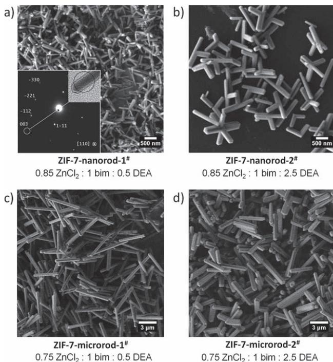
**Figure 3.** a–d) SEM images of the ZIF-7 nanorods and microrods. Inset in (a): Typical SAED pattern from a single nanorod (ZIF-7-nanorod-1<sup>#</sup>), verifying that the long axis of the rod-shaped crystal is parallel to the *c*-axis. The image descriptions give the molar ratios in the synthesis solutions.
