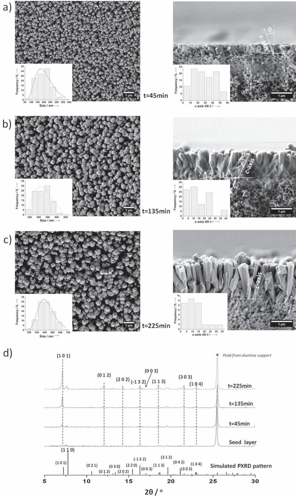
**Figure 4.** SEM top views and cross sections of the ZIF-7 membranes obtained after different times of microwave assisted secondary growth: a) 45 min, b) 135 min, and c) 225 min. d) the XRD patterns of the ZIF-7 membranes and the simulated PXRD pattern of ZIF-7 crystal. Insets in the SEM top views give the distributions of the cross-sectional size of the columnar crystals, and the CPO distributions. The CPO is represented by the angle  $\theta$  between *c*-axis and the substrate normal.
