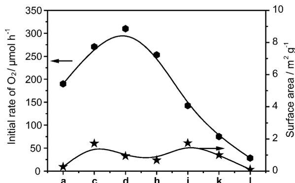
Figure 11. The rate of  $\text{O}_2$  evolution and surface area of  $\text{BiVO}_4$  samples synthesized by adding different amounts of  $\text{TiCl}_3$  as directing agent and adding optimum amount of  $\text{TiCl}_3$  under different pH values. Reaction conditions: catalyst, 0.3 g; light source, 300 W Xe lamp with cutoff filter;  $\text{AgNO}_3$  solution, 0.05 M, 200 mL.
