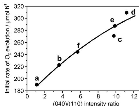
Figure 8. The correlations of the oxygen evolution rate with the (040)/(110) intensity ratio in the XRD patterns of the corresponding samples  $\text{BiVO}_4$ -a-f. Reaction conditions: catalyst, 0.3 g; light source, 300 W Xe lamp with cutoff filter ( $\lambda \geq 420$  nm);  $\text{AgNO}_3$  solution, 0.05 M, 200 mL.
