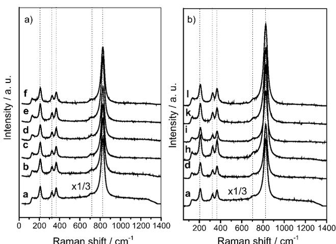
Figure 7. Raman spectra of a)  $\text{BiVO}_4$  synthesized with different concentrations of directing agent by molar ratios of  $\text{BiVO}_4$ -a-f and b)  $\text{BiVO}_4$ -a and the  $\text{BiVO}_3$  samples synthesized with the optimum amount of directing agent under different pH values:  $\text{BiVO}_4$ -d, h, i, k and l.
