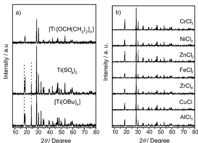
Figure 2. XRD patterns of a) the  $\text{BiVO}_4$  samples synthesized with different Ti-containing precursors as the directing agent and b) the  $\text{BiVO}_4$  samples synthesized with different chlorides as the directing agent. The characteristic peaks of the tetragonal  $\text{BiVO}_4$  are indicated by a dotted line when  $\text{Ti}(\text{OBu})_4$  and  $\text{Ti}(\text{SO}_4)_2$  were used as Ti-containing precursors.
