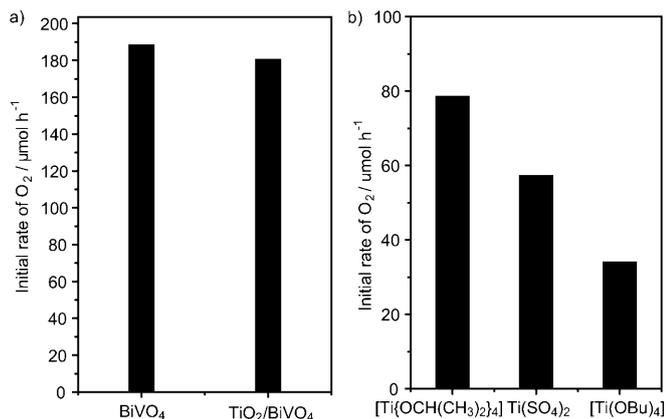
Figure 10. The initial rate of  $\text{O}_2$  evolution over a)  $\text{BiVO}_4$ -a and  $\text{BiVO}_4$ -a doped with  $\text{TiO}_2$  by impregnated method photocatalysts and b)  $\text{BiVO}_4$  samples synthesized with Ti-containing precursors as directing agent from an aqueous silver nitrate solution under visible-light irradiation ( $\lambda \geq 420$  nm). Reaction conditions: catalyst, 0.3 g; light source, 300 W Xe lamp with cutoff filter;  $\text{AgNO}_3$  solution, 0.05 M, 200 mL.
