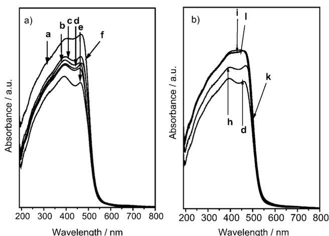
Figure 6. UV/Vis diffuse reflectance spectra of a)  $\text{BiVO}_4$  synthesized with different concentrations of directing agent,  $\text{BiVO}_4$ -a-f and b)  $\text{BiVO}_4$  synthesized with the optimum amount of directing agent under different pH values:  $\text{BiVO}_4$ -d, h, i, k and l.
