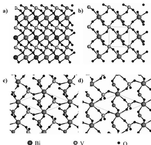
Figure 12. a) Vertical view of the surface atomic configurations for the (040) facet in monoclinic  $\text{BiVO}_4$ . The slab system of b) the (040) facet, c) the (110) facet and d) the (011) facet in the monoclinic  $\text{BiVO}_4$  primitive cell after geometry optimization.
